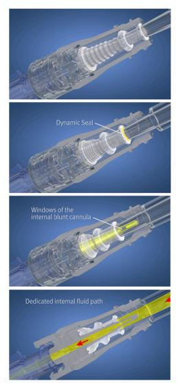
When the MicroClave does not have a male end connected, the split septum seals the cannula, maintaining neutral displacement and does not allow contaminants to enter the port
